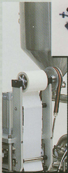
MODEL NB070-BIS Fully Automatic Filling & Sealing Machine Output up to 60 CPM
