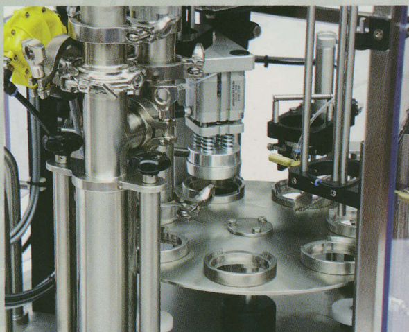
MODEL PLF-5SA/B Semi-automatic Filling & Sealing Machine Output up to 15 CPM
